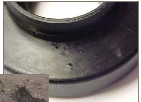
Pitting on filter end-cap
