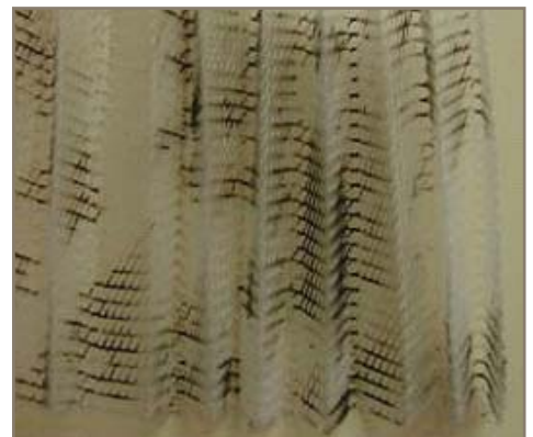
Burnt polymer pleat support mesh from arcing
