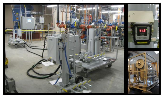
High Purity Northwest provides procedures and specifications, flushing and filtering equipment and on site particle testing to complete oil flushing procedures within hours rather than weeks of flushing.
