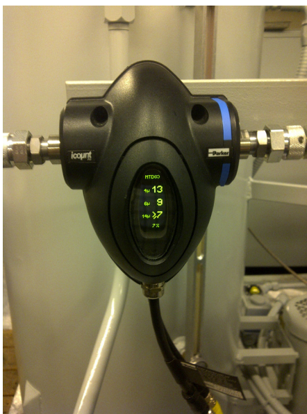
Online Laser Particle Detector - ISO4406:99, NAS 0-12 & Moisture in %RS all in One Device
