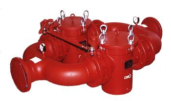
The Series 530/531 is a compact unit, in-line inlet/outlet connections, which enables easy piping and variable strainer placement. Chamber change over is accomplished quickly and easily. A single lever controls the positive sealing butterfly valves, changing the fluid flow.
