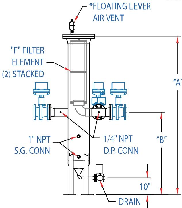
\*Floating lever air vents are for liquid units.
