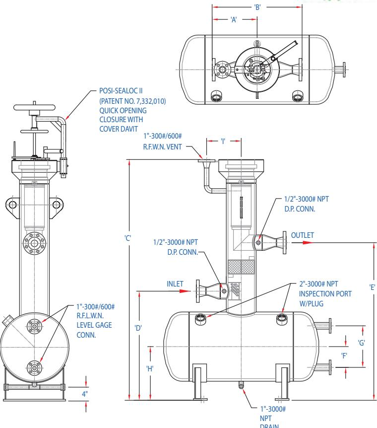
\*Note: 2" & 3" have concentric reducer on inlet and outlet.
