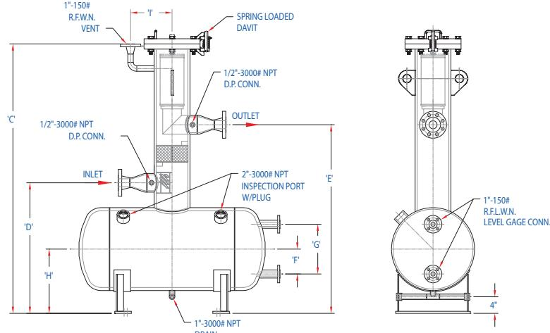
*\*Note: 2" & 3" have concentric reducer on inlet and outlet.
